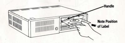
Turn the diskette-slot handle to the *closed* (vertical) position.
