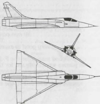
The *Mirage 2000* is an old but popular French-built export fighter. The large delta wing is lightly loaded, and produces high drag in maneuvers, losing velocity quickly. It can perform intercept and ground attack missions. It is slightly better than a MiG-21 in a dogfight.
